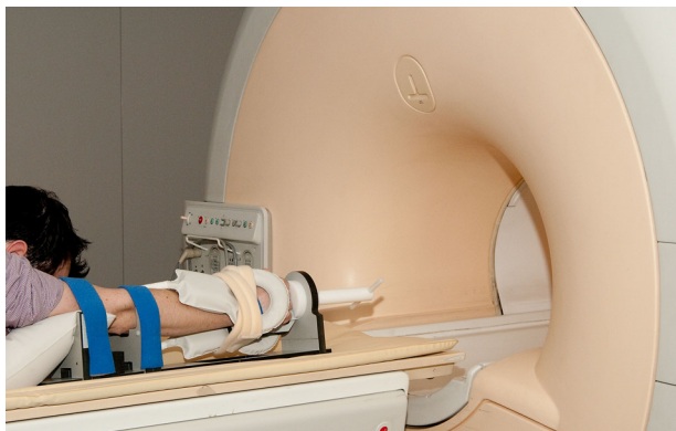
Figure 1. MRI jig in use in the 3-T MRI scanner in the 'superman' position. Standard MR coils can be seen strapped to the wrist.
